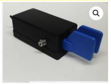
The CW paddle is commercially available from Gigaparts & others. It is printed off on a 3D printer, and works well for the price point (\$42).
