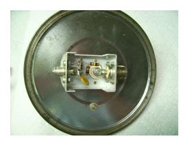
Top of the can is a diode RF detector used to sample the amount of RF present
