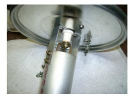
Top of the 50 ohm resistor connection to the RF output circuitry above the lid
