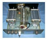
Note on the left picture, there is only 1 insulated connector for a long-wire. The front panel antenna switch shows a balanced line choice. This is possible only by using an external 1:1 or 1:4 Balun. This company made other model tuners with a built-in Balun and had 2 white ceramic insulators on the rear panel.
