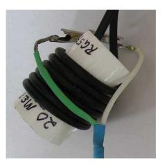
The adapter in use checking a 20 meter trap. The clips are connected together, forming a loop.
