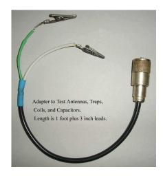
A homemade adapter for checking antennas as well as traps and resonant circuits.
