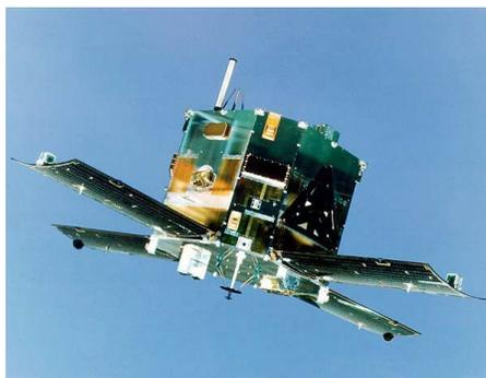
Communications Package is anticipated. The Intelsat geosynchronous platform would be able to provide the AMSAT Phase IV Lite payload with approximately 400 Watts of DC power for 15 years.
